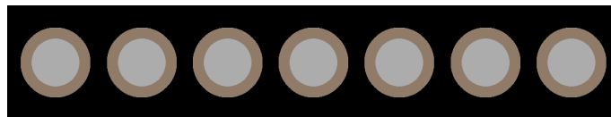
Non Plated Hole (Slot separator)
