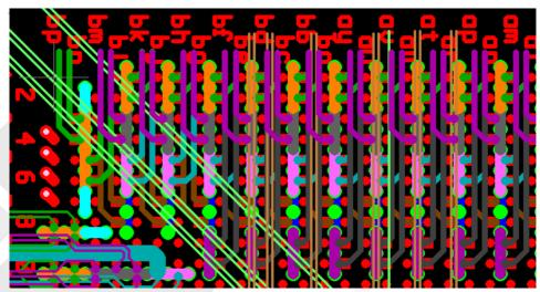
In the image above you can see that we run traces from the banks through this section. The SI engineer needs to determine if this is acceptable. The layers are all shielded and the connections will not penetrate the layers below.
