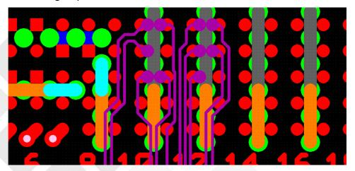
We are using 0,1mm trace width and 0,1mm spacing for the bank section. This will yield a 5 trace routing channel on its most critical position. Further in this document we show the exact design rule dimension of the complete structure.
