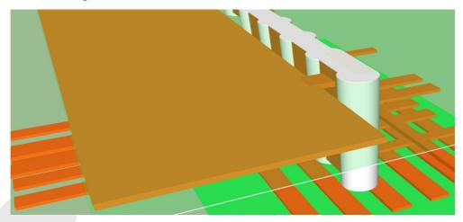
The following images show how we use VeCS-2 technology in a array construction. These images show also the advantage, not penetrating all layers creates huge amount of routing space. This is the same as Microvia/Anylayer technology with the difference that we do not need sequential lamination process for fabrication but use a single lamination cycle.
