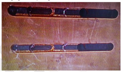
The technology for creating the VeCS-2 slot as used in this application is a 0,5mm slot. This wider slot gives us the ability to clean the bottom to split the slot in two parts creating 2 high-density connections. The width of the separation is 0,3mm.
