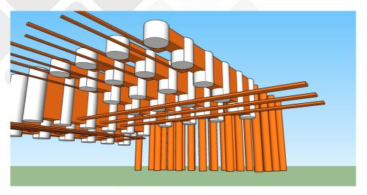
As shown in the image above as we go closer to the centre of the BGA we step further down into the board. We can even combine it with a section going all the way through the board. Many combinations are possible.
