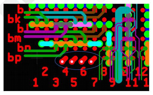
As the previous image is shown we have 4 dog bone via connections to non critical signals. VeCS can be used as well but we want to demonstrate that VeCS and traditional technology can be mixed.
