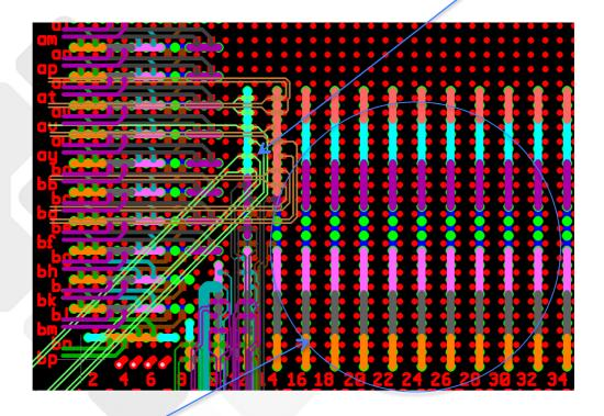
On the right hand side you see the slots represented in different depths. We have a total of 7 different depths for a total of 7 signal layers. As 7 layers would not be a good balance we propose to use 8 signal layers. The slots are all stepped down from low to high but we this is not a
