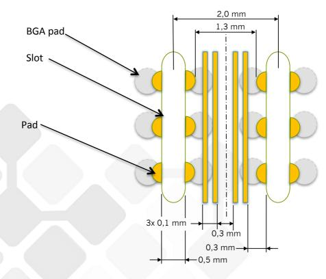
As an alternative we can run a single differential pair between the slots as shown in the following example reducing the DC loss of the pair.
