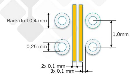
To increase the separation between the back drill and the traces the drilled hole size is reduced to 0,2mm in order to reduce the back drill diameter to 0,35mm and increase the trace to back drill spacing.
