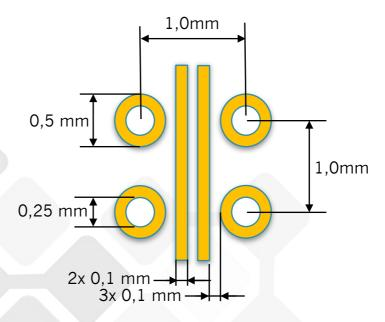
The back drill design rule is shown in the following section.
