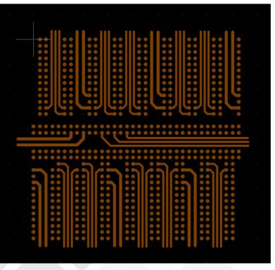
The ground or power layer is shown below in reverse. No connection to the VeCS are shown. These can be added by adding a trace. The slot to plane spacing used here is 0,15mm.
