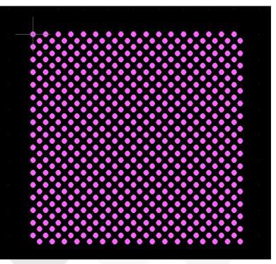
First internal layer (L2) with landing pads for the microvias and the redistribution to the VeCS slot.
