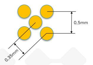
With current through hole technology routing this device is not an option. Using Microvias is an option but the pad sizes for Microvias are for advanced technology 0,2mm which means a routing channel in the 0,35mm direction of 0,15mm. This yields a track and gap of 0,05mm.
